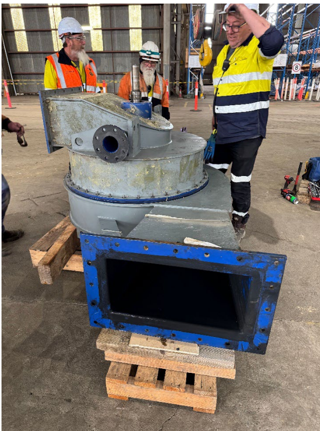
Disassembly of the Spray Roaster's gas transport fan to complete coating repairs
