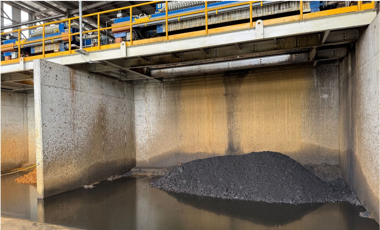
Successful production of Char/Silica wet filter cake by-product during operations.
