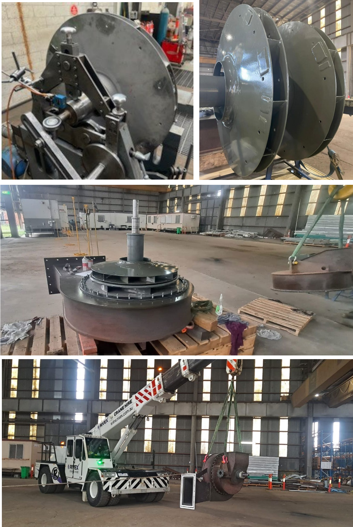
Figure: Impellor pre & post coating, dynamic balancing and completed gas transport fan assembly ready for installation and commissioning.
