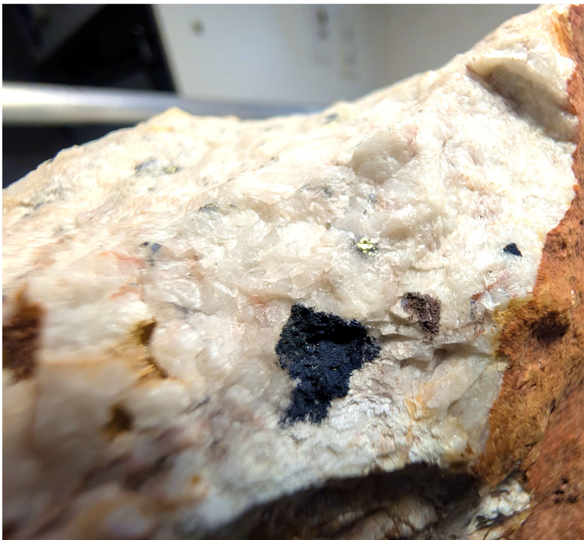
Figure 2. An example of copper mineral bornite - yellow (fresh) and deep blue (oxidised) from sample 25RC0148 (2680ppm Cu). The large oxidised bornite grain is approximately 8mm wide.
