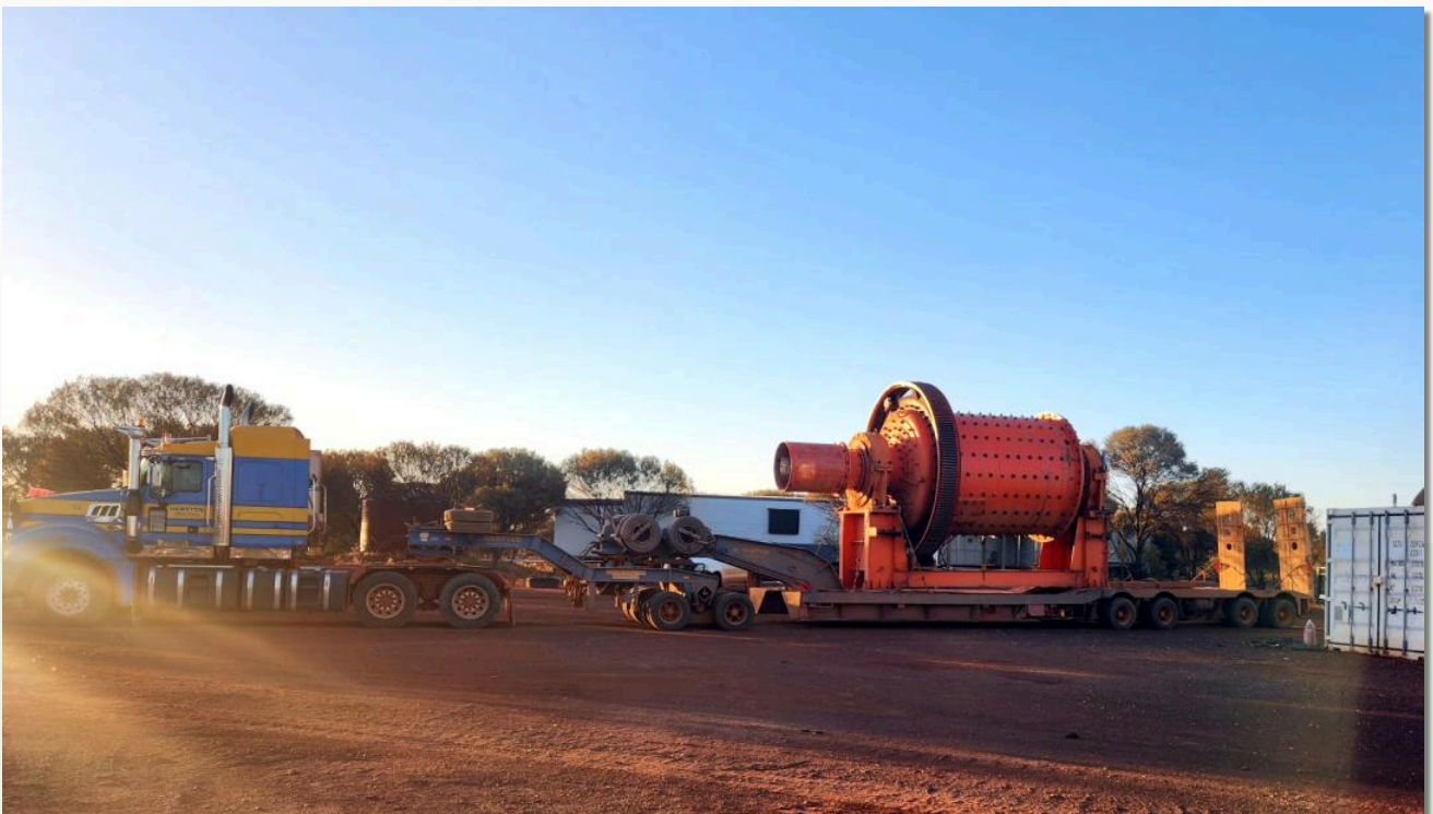
Picture 1: Ball Mill during relocation
