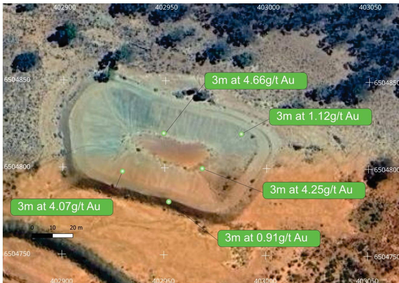
Figure 5: North East Tailings Dam Drilling Results (Pre-Relocation)
