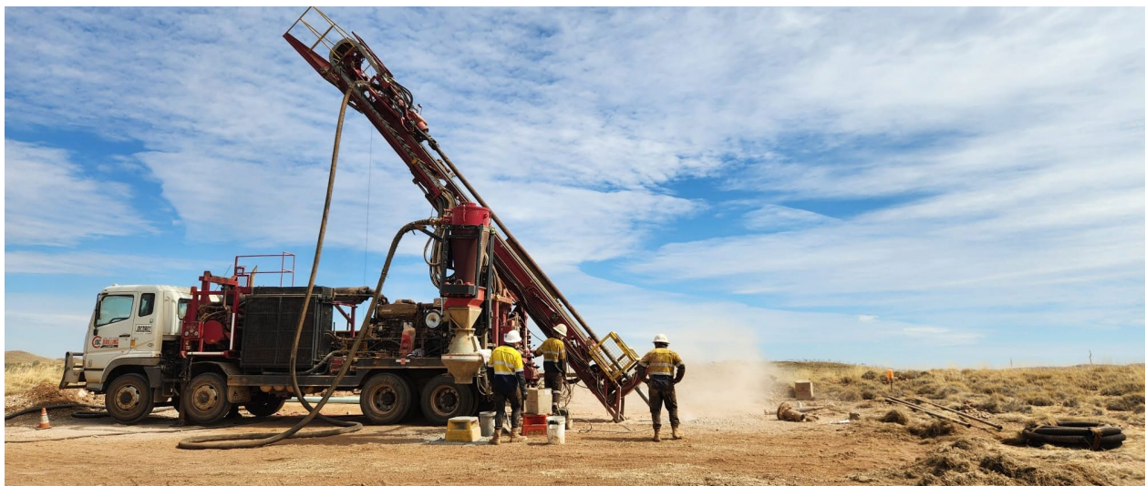
Figure 1: Drilling contractor JDC collaring the first hole of MBG’s Phase 2 drill program at site.
