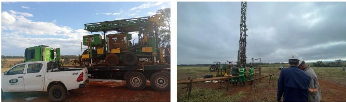
Figure 6 - Rig mobilisation (left) and diamond drilling operations (right) supporting the expanded Piracanjuba field programme. Photographs provide operational context only and do not report Exploration Results.
