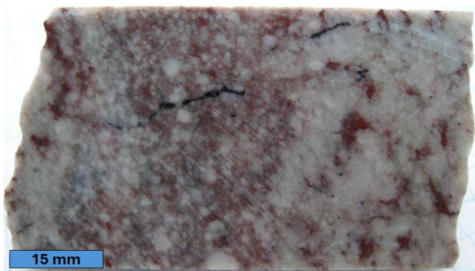
Figure 3: Sectioned dolomite-carbonatite (BD-Zone) core showing ~1-2 weight % REE-fluorocarbonate mineralisation. Other minerals include ~94% dolomite, ~2% apatite, ~1% biotite, and ~1% fluorite.
