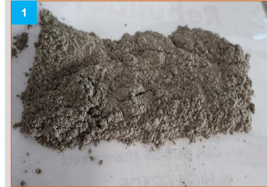
1 Pulverised spent catalytic converter feedstock rich in PLATINUM GROUP METALS (Palladium, Platinum, Rhodium)
