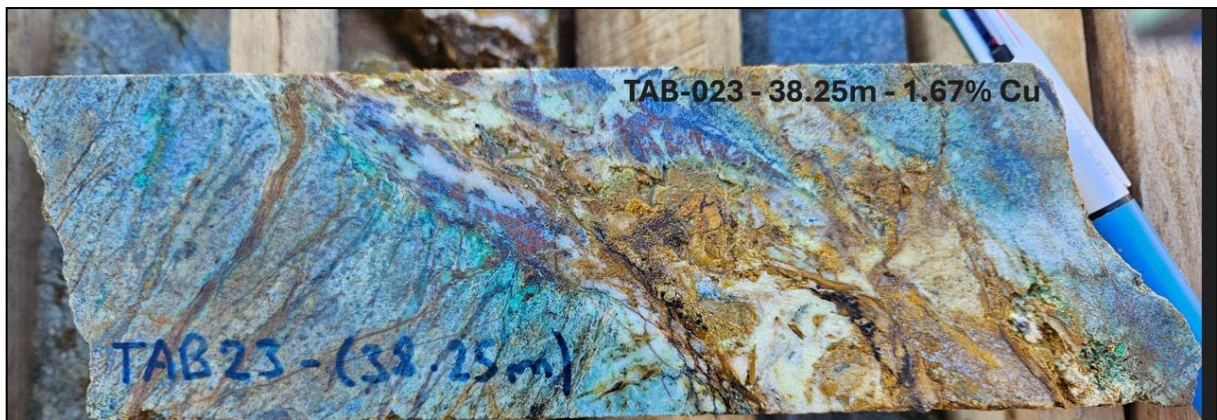
Image 5**: TAB-023 showing typical sulphide mineralogy to be re-assayed for CuT and Au
