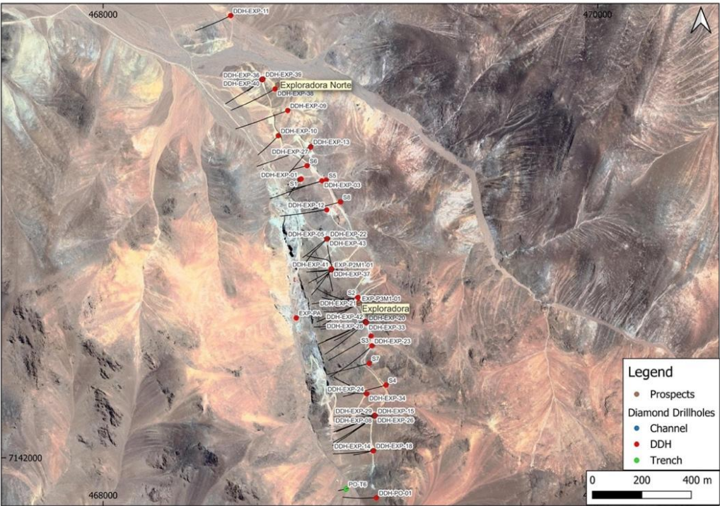
Figure 5: Exploradora Project Drill Collar and Trench Plan
