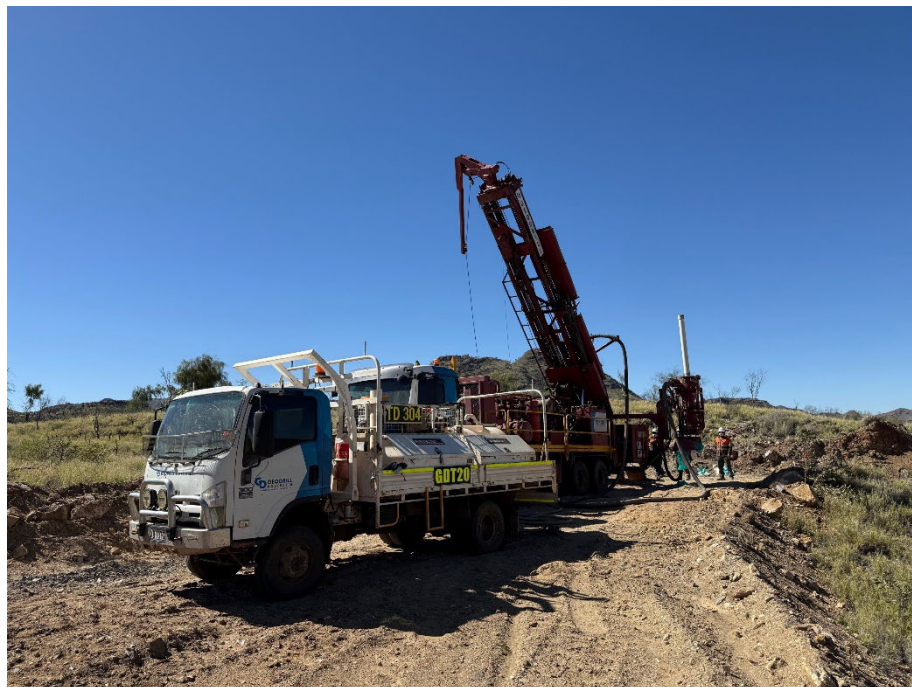
Figure 2: GeoDrill reverse circulation drill rig at Harts Range
