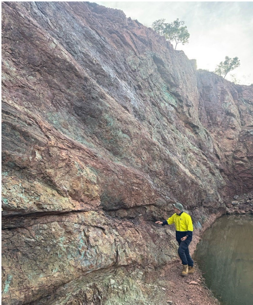
Figure 1: Jointing and shearing displayed along face of Pit 1 at the Big One Deposit
