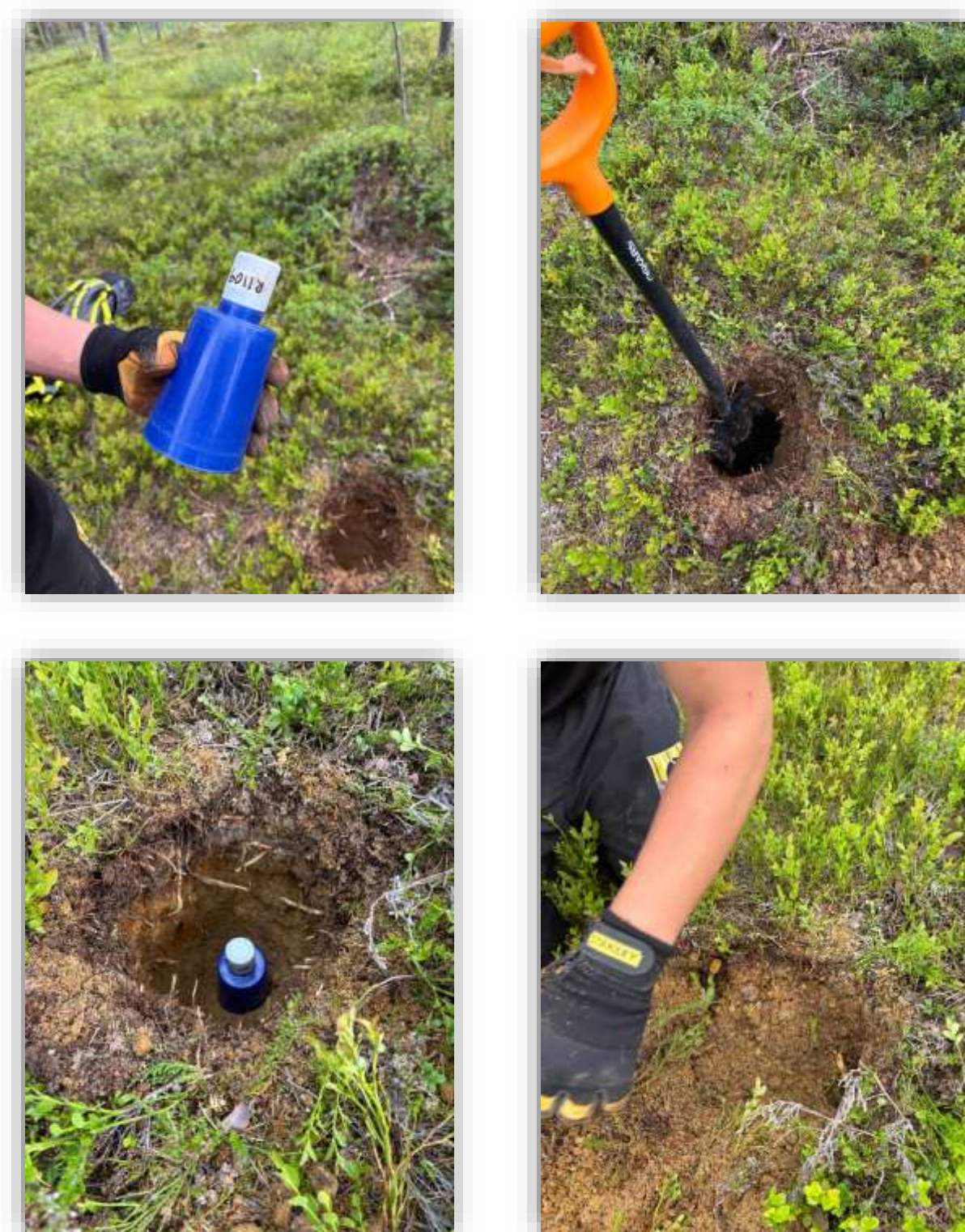
Figure 3: RadonX™ field deployment. Each inverted detector cup is buried in a shallow hole, with its location recorded by GPS and marked with flagging tape. The detector is recovered approximately 10 days after deployment for field analysis.
