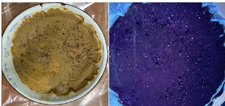
Figure 2: Left: Knelson concentrate under natural light. Right: same concentrate under UV light, showing fluorescent scheelite.
