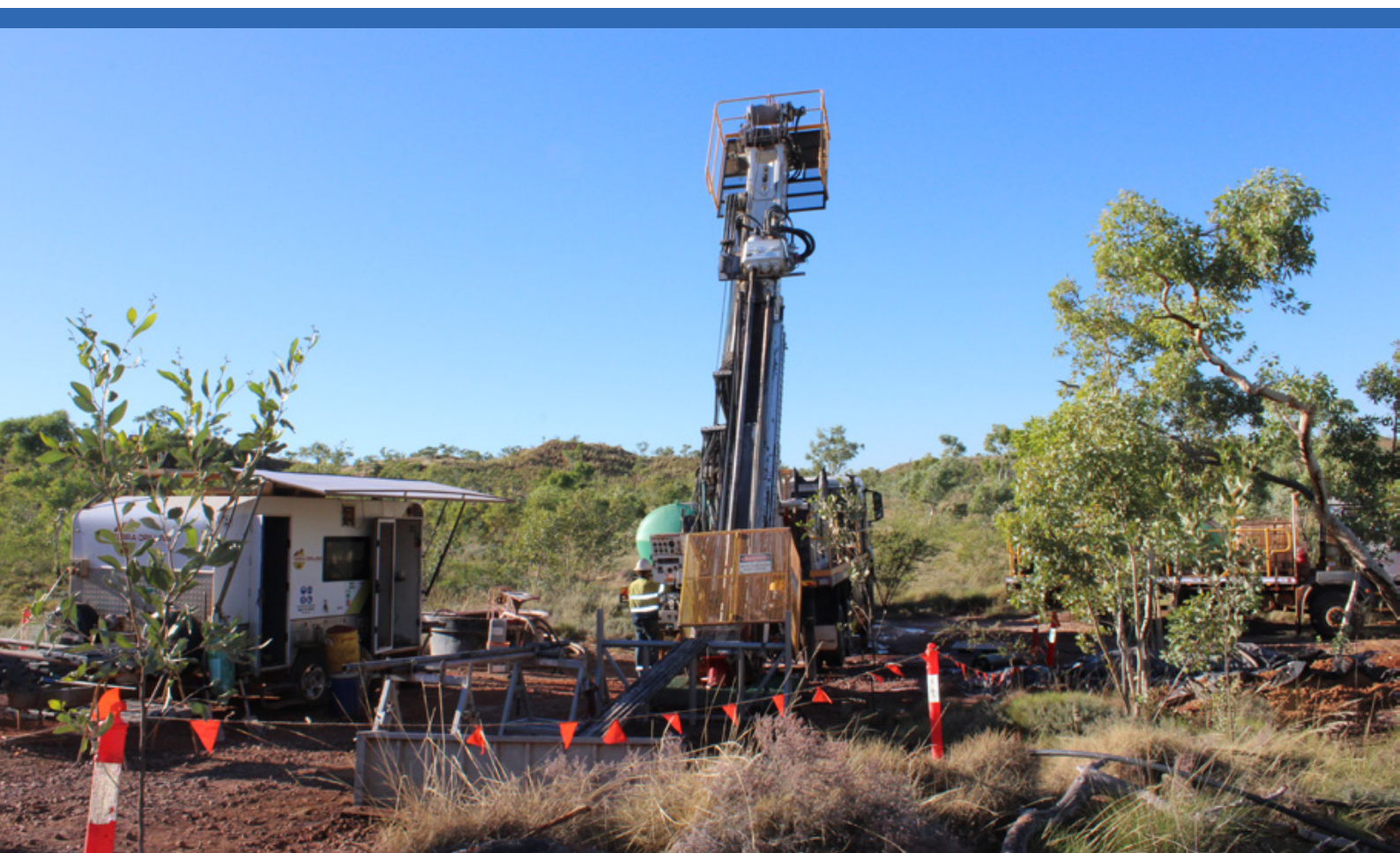
FIGURE 9 Diamond Drilling at Gambit East Deposit.
