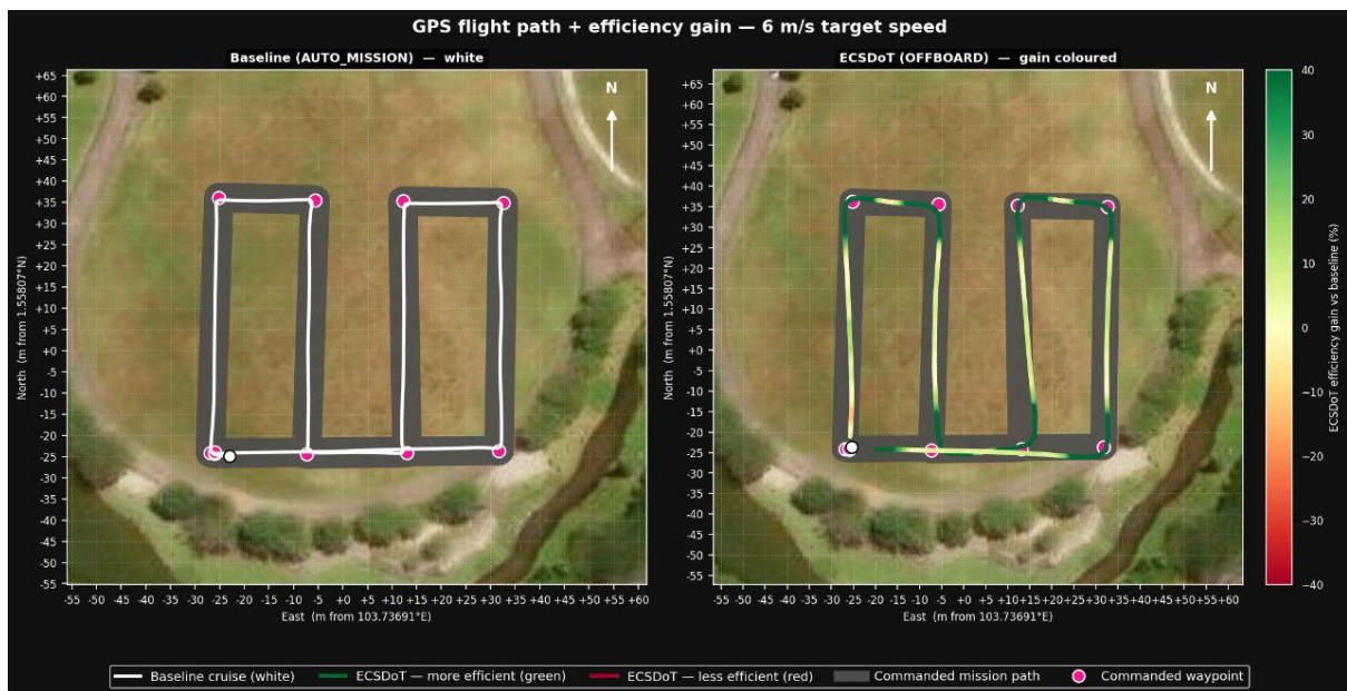
Figure 6: GPS Flight Path Efficiency Overlay at 6 m/s - Baseline (White, Left) vs ECS-DoT Efficiency Gain (Colour-Coded, Right)
