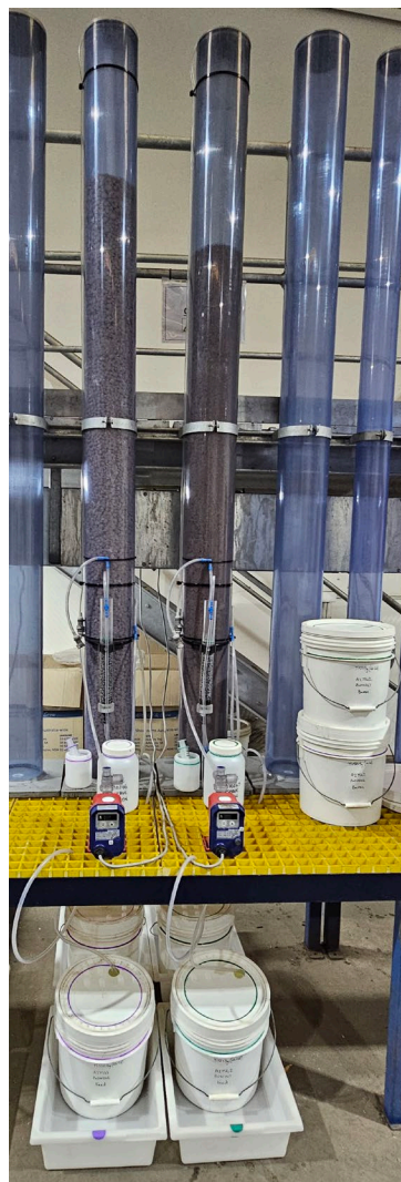
Figure 6 – ALS Laboratories Oxide (HW) and Transition (MW) column leach test setup.
