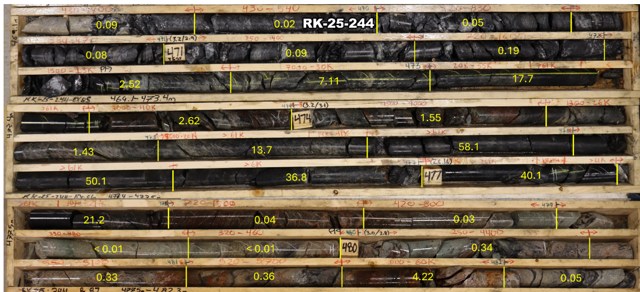
Figure 3: Core photo with assays from RK-25-244, grades are shown as % U_3O_8
