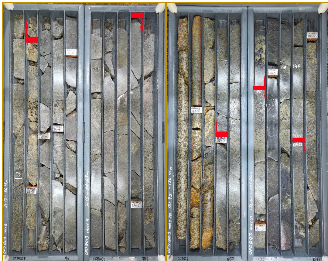
Figure 18. Sweeneys Drillhole OFD003 Core Tray showing granite host rocks with sulphide lodes observed at depths of 33.55 – 39.80m and 135-139.55m.
