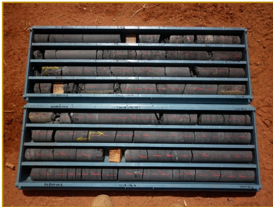
Figure 12. Byro Core Tray (Drillhole 24BDD002 Depth 7.2 – 14.15m) showing Permian Black Shale (refer ASX announcement 25 February 2025)
