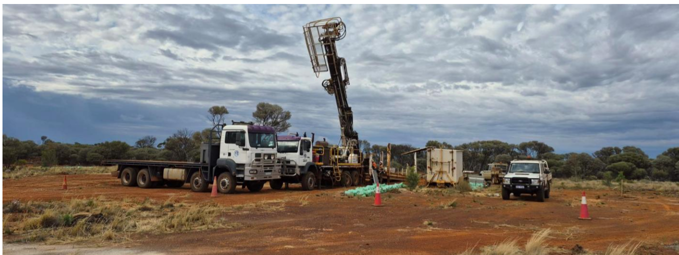
Figure 1: Diamond drilling James Stage 1 metallurgical testwork hole
