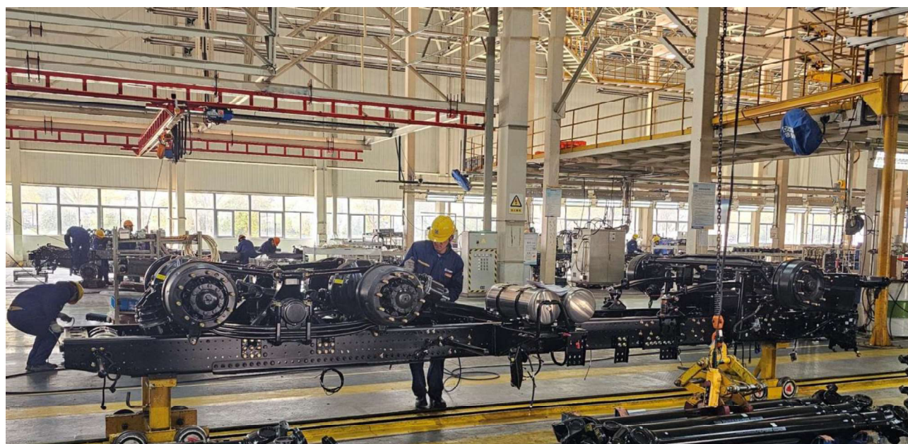
Image 3: Drive trains assembly being reviewed
