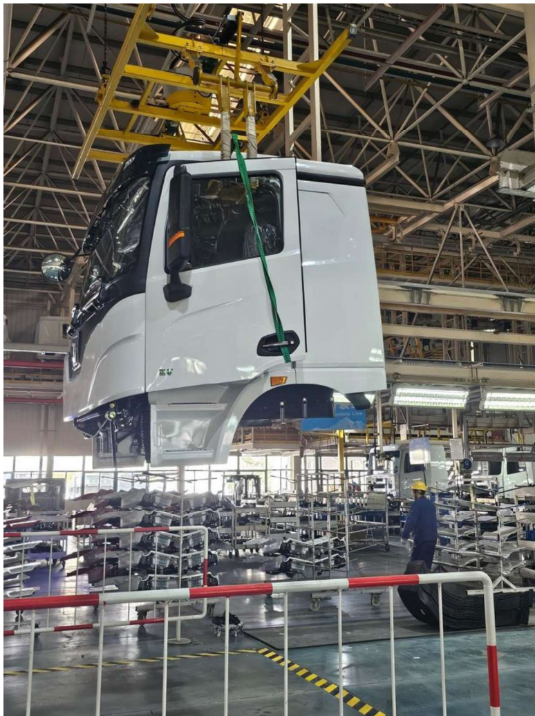
Image 1: Driver cab assembly in progress for a battery-swap enabled rigid truck at manufacturing facility
