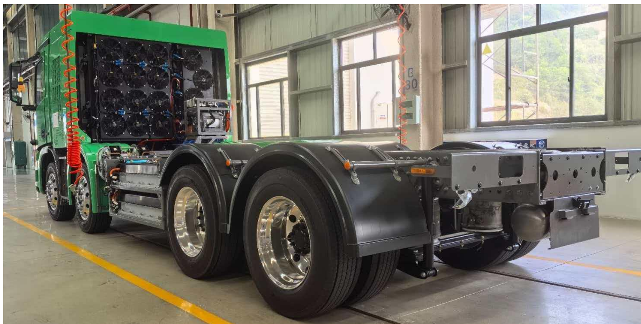
Image 2: Rear view of the HFC 8x4 32T concrete agitator truck for Heidelberg Materials
