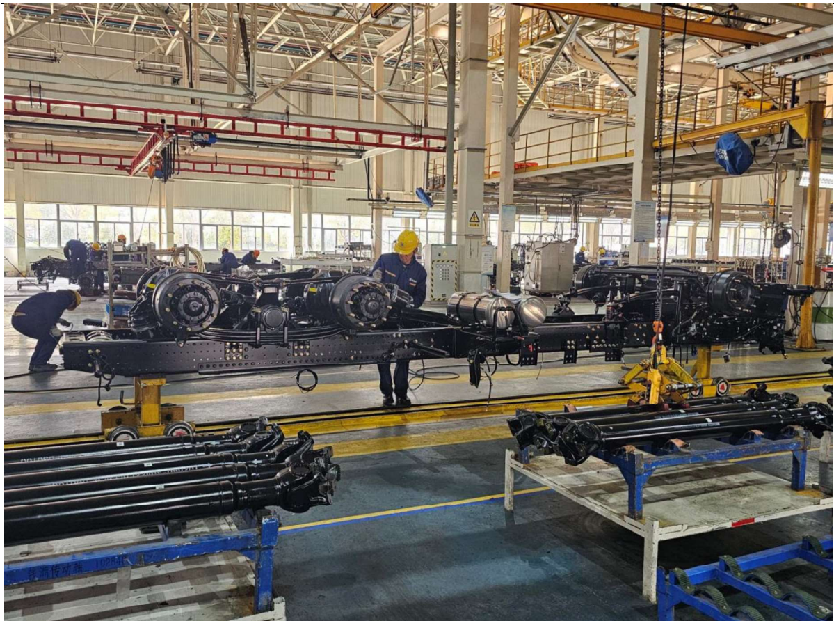
Drive trains assembly being reviewed
