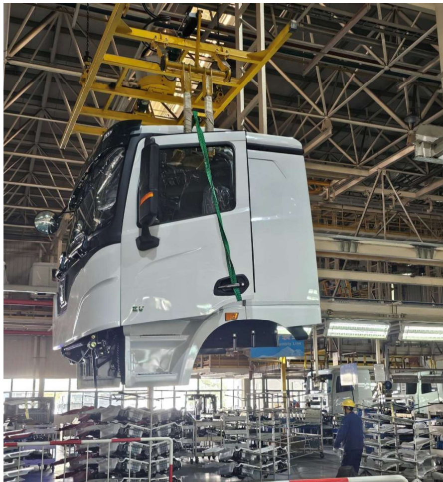
Driver cab assembly in progress for a battery-swap enabled rigid truck at manufacturing facility
