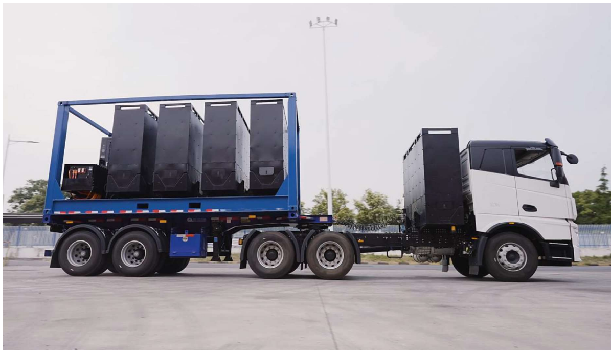
Image 1: Alpha battery-swap electric prime mover
