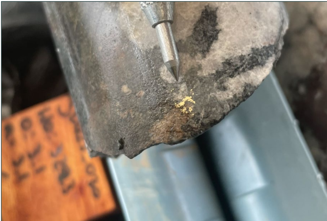
Figure 4 -SDH25-030, 329.2 meters down hole, visible gold in Hematite-magnetite matrix
