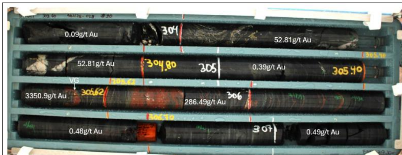
Figure 2. SDH25-028, 305.4 - 306, He-Mt alteration and high Au grade
