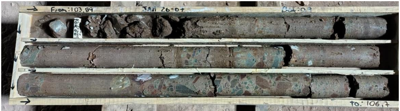
Figure 1. JAM 25-07 core sample 103m to 106m gravels and sand contributing to high porosity – packer test done on this interval
