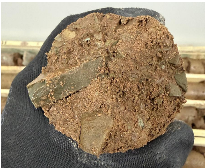
Figure 5. Section from failed packer test interval showing sandy clay units with large shale fragments.
