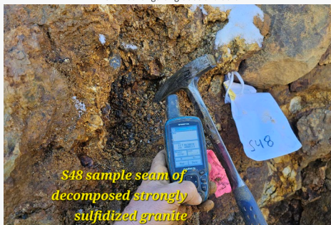
Photo showing sample S48 at Springfield Prospect, here we see strongly oxidised sulphides in granite which returned 7.75 g/t Au and 0.1% WO3
