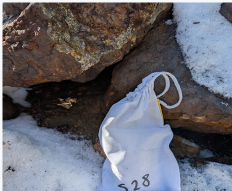
Picture showing sample S28 with massive pyrrhotite associated with tungsten mineralisation. Sample 28 returned tungsten grades of 0.96%
