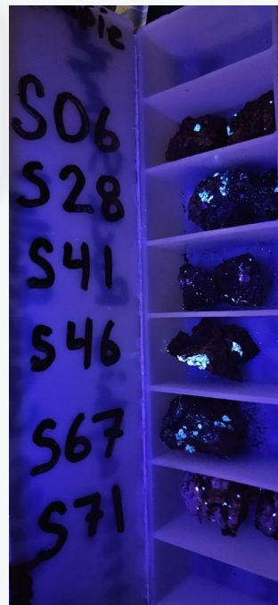
(left) Image showing scheelite mineralisation under short wave UV light in samples selected for petrographic analysis (right) Image of S28 showing massive Pyrrhotite at Springfield associated with tungsten mineralisation.
