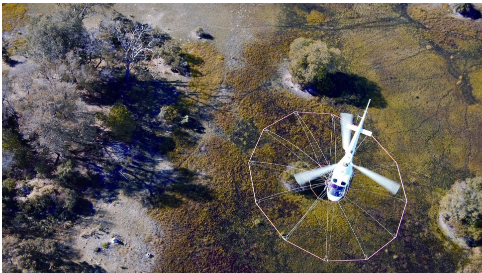
Figure 5: Example photo of airborne VTEM system used by GEOTECH to complete the VTEM survey at Springfield.
