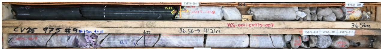
Figure 5: Massive pollucite mineralization in drill hole CV25-975 from the Helio Zone . Core grades 1.0 m at 21.52% \text{Cs}_2\text{O} (36.5 m to 37.5 m).
