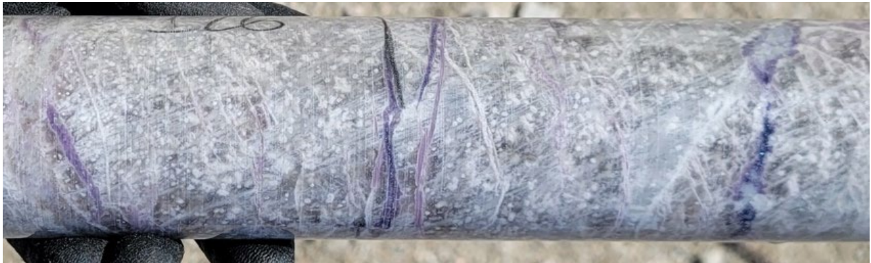
Figure 2: Pollucite with late stage lepidolite (purple) and spodumene/pollucite (white) veining displaying classic “tapioca” texture (white blebs) at a depth of ~126 m in drill hole CV25-948 from the Vega Zone . Core grades 1.9 m at 17.81% Cs 2 O (125.0 m to 126.9 m) within a wider mineralized interval of 28.0 m at 8.05% Cs 2 O (116.5 m to 144.5 m)
