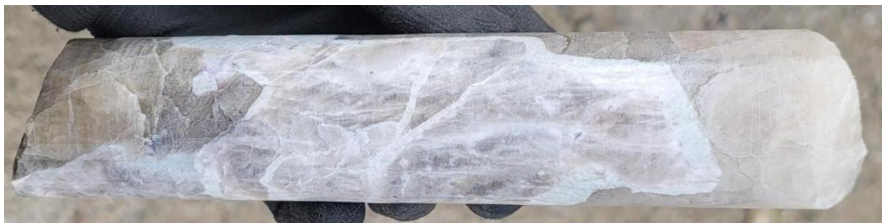
Figure 2: Pollucite with late stage spodumene/pollucite (white) veining displaying classic “tapioca” texture (white blebs) at a depth of ~43.7 m in drill hole CV25-979 from the Helios Zone . Core grades 0.5 m at 2.33% \text{Cs}_2\text{O} within a wider mineralized interval of 4.9 m at 3.65% \text{Cs}_2\text{O} (39.0 m to 43.9 m)
