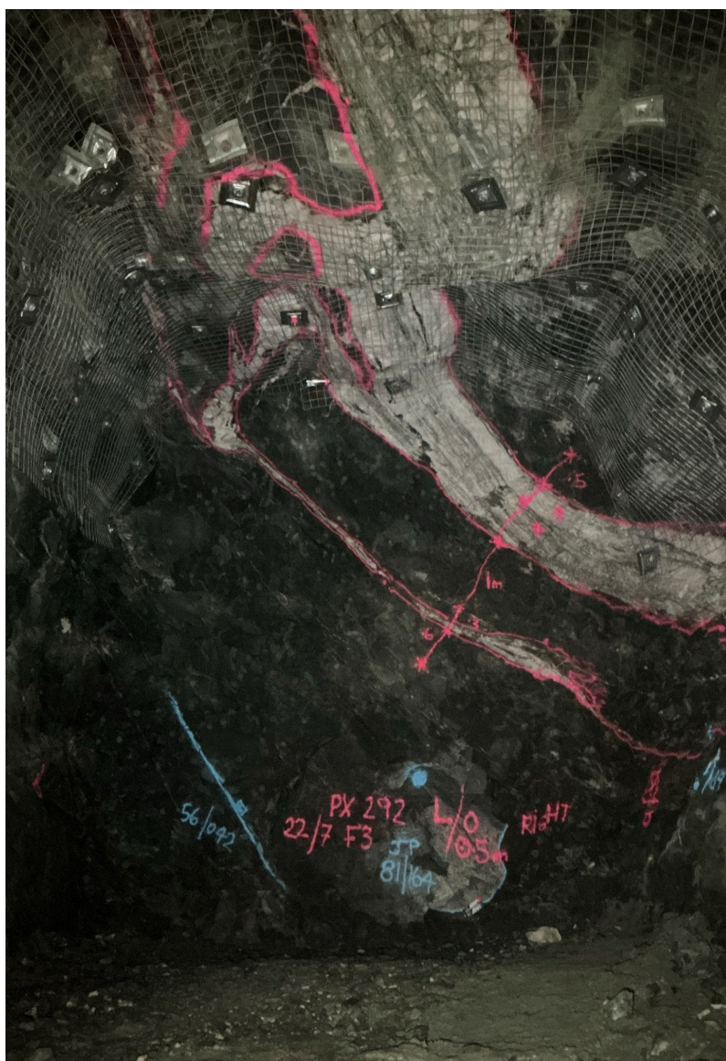
Photo: Development ore face with HG laminated Mararoa Reef from the in ore ramp on the Phoenix pillar.
