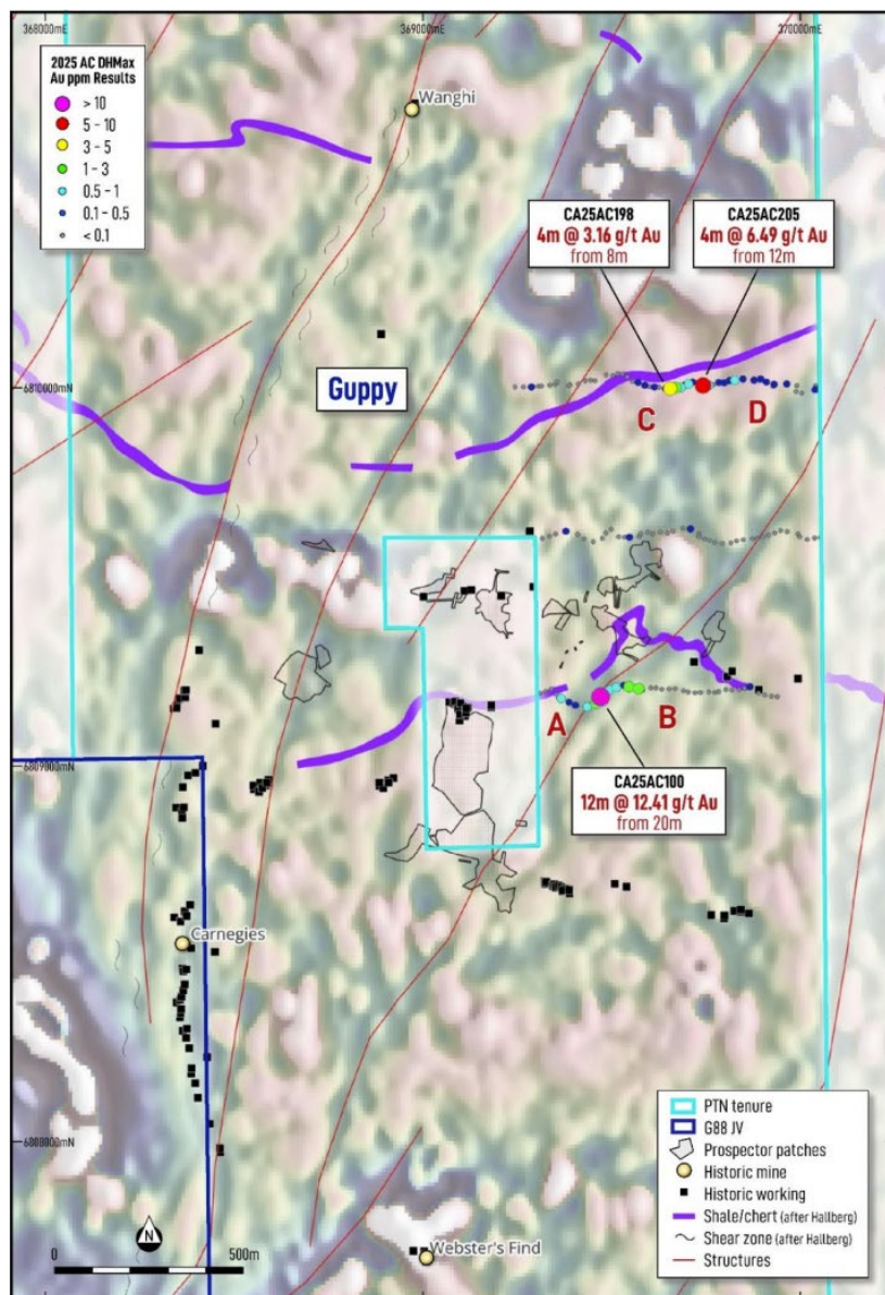
Figure 4: Guppy prospect air-core holes by DHMaxAu, associated with chert/ironstone lithologies, and possible D1 NE-SW trending structures interpreted from aeromagnetics. Numerous historic and more recent 'scrape and detect' prospector workings highlight the local gold endowment.
