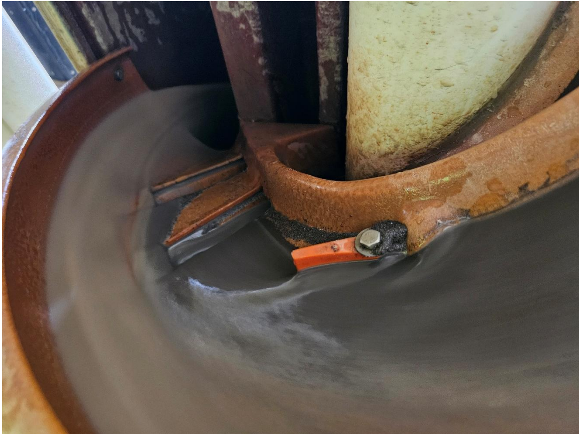
Photo 1: Rosewood HM sample being feed through a wet spiral separator at IHC Laboratories. Darker HM minerals on inner side of the spiral are split off as part of the HMC concentration process, September 2025.
