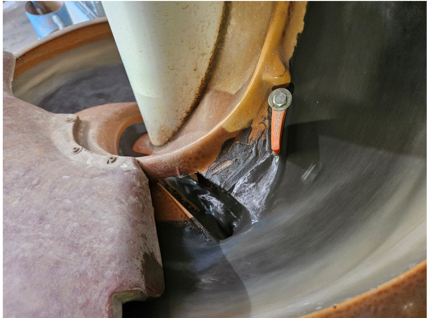
Rosewood HM sample being feed through a recleaner spiral at IHC Laboratories.
