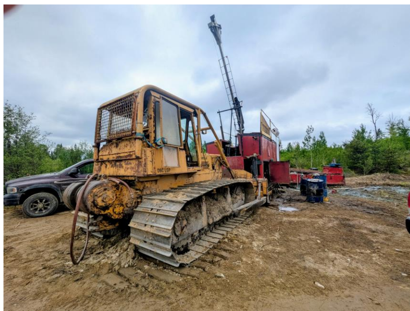
Figure 4: Diamond drill rig at the Shanty Lake target, where the bit is approximately 150m from target.
