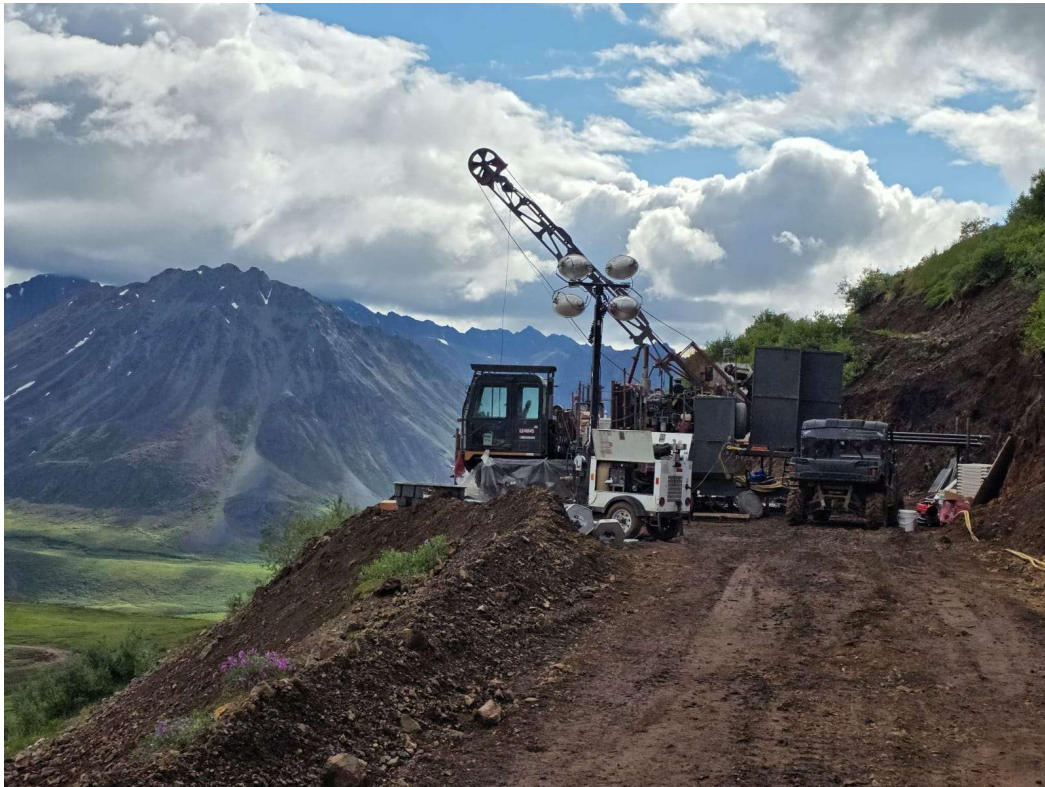
Figure 1. Diamond drill rig undertaking oriented diamond coring at Caribou Dome (CD25-001)
