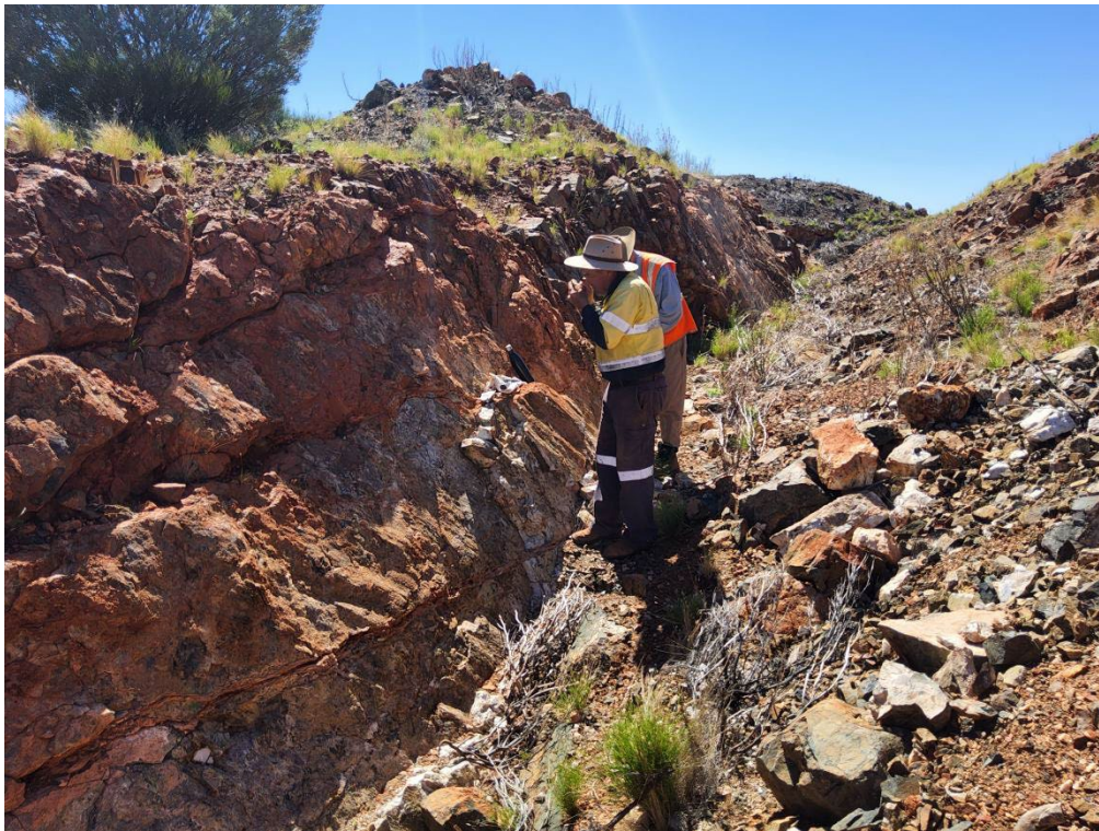
Figure 20. Kilkenny Workings – Field photograph showing historical costean, north wall oriented E-W, looking east, exposed sheared mafic rocks with quartz veinlets observed in sheared mafic rocks. Geological observation only; no assays are associated with this photograph. (MGA94 Z51 - 386600mE 6792215mN)
