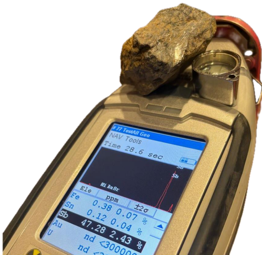
Figure 1: High-Grade Stibnite mineralisation sample 733655 (45% Stibnite Visual Estimate) located at Easting 596828 and Northing 5265334 NAD 1983 Zone 11, with the pXRF reading of 47.3%.
