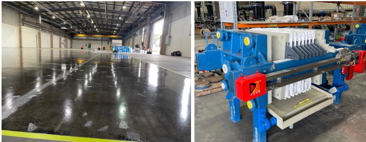
Figure 1. Site preparation works at PSG demonstration facility in Adelaide (left) and filter press at laydown facility in Adelaide (right)
