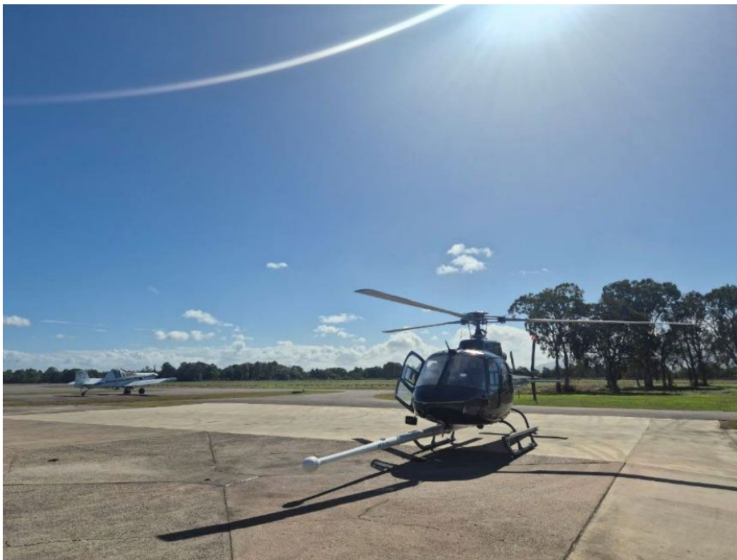
Figure 2 – ASX 16/06/26: Helicopter with magnetometer stinger at Ingham, northeast Queensland.
