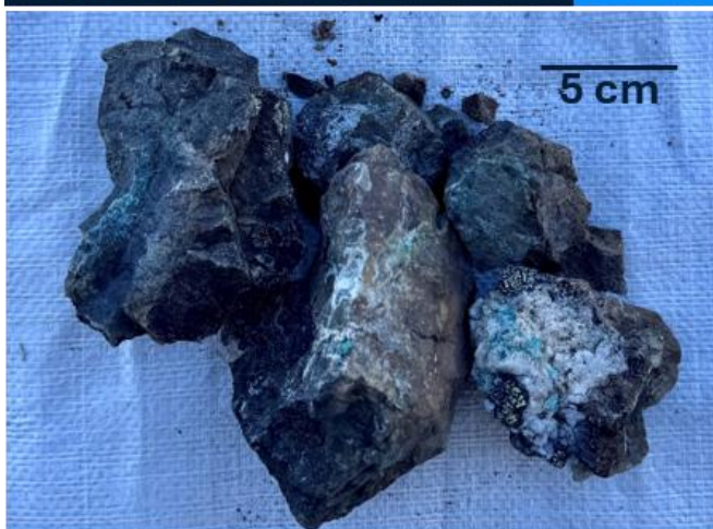
Figure 1: Selected surface rock chip samples, Talisker Central and Talisker South, showing copper mineralisation. Assays pending. Refer to the cautionary statement on visual estimates of mineralisation within this announcement.
