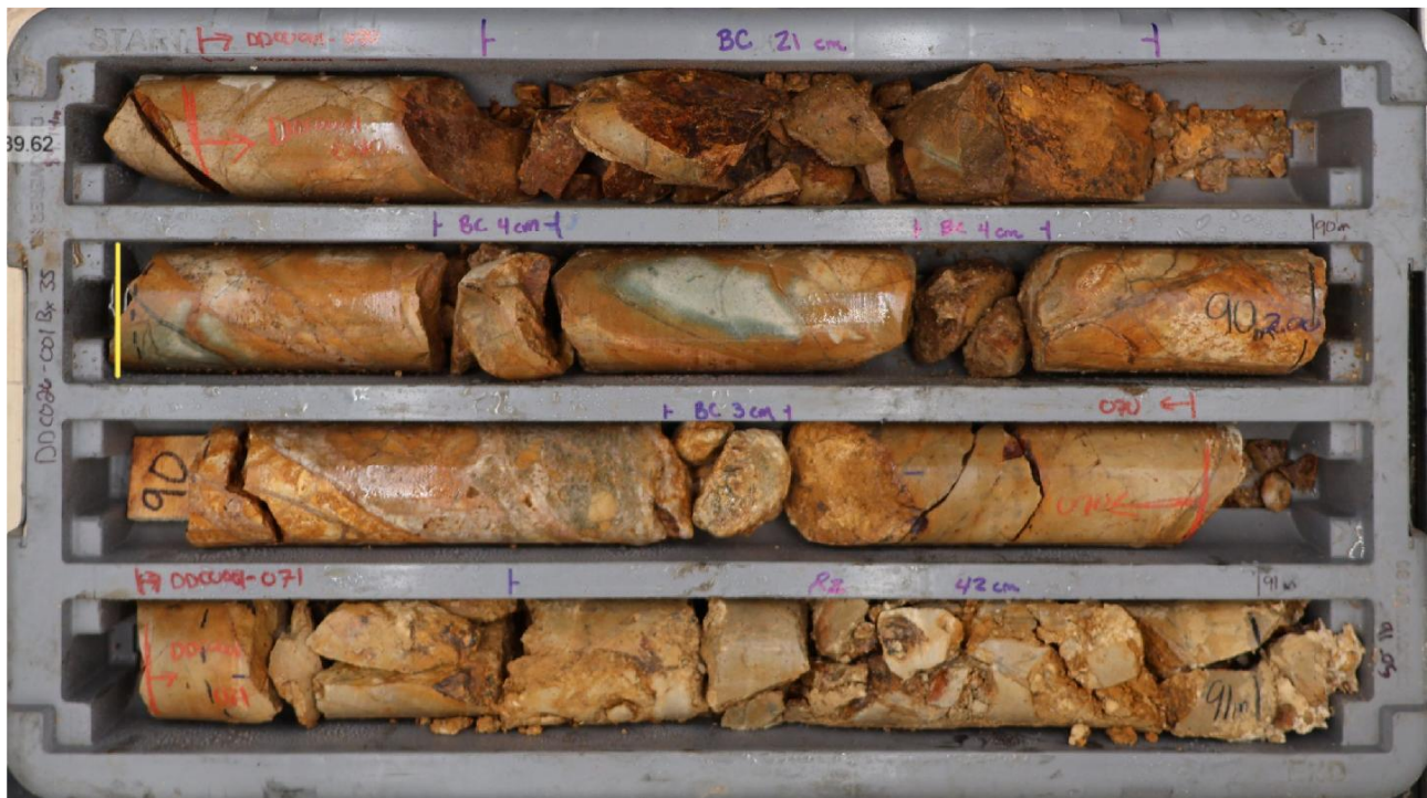
Figure 3: Representative drill core from DDCO26-001 (89-91m). Near-surface oxidised material: note argillic alteration, quartz-chalcedony veining, and vugs with iron staining after oxidised sulphides. Visual observations only; not a proxy for grade.
