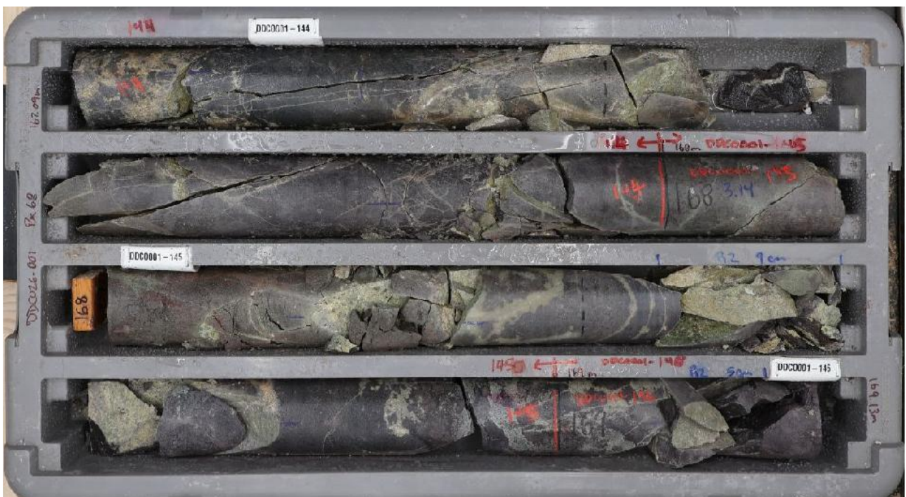
Figure 4: Representative drill core from DDCO26-001 (167-169m). Deeper fresh (unoxidised) material: note lower alteration intensity, quartz-chalcedony veining, very competent without iron staining as sulphides are unoxidised. Visual observations only; not a proxy for grade.
