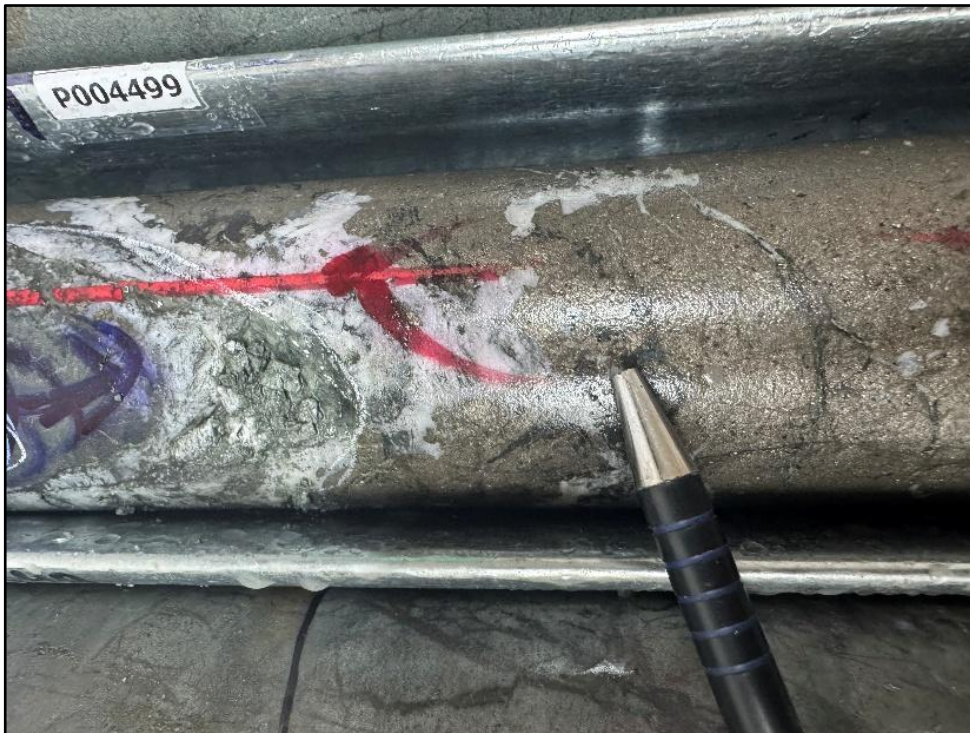
Figure 5. Core photo showing carbonate replacement pyrrhotite-pyrite-sphalerite-galena mineralisation in ZRPD25004 from 848.4 to 849.9m – 5.1% Pb, 2.1% Zn, 32.6g/t Ag.
