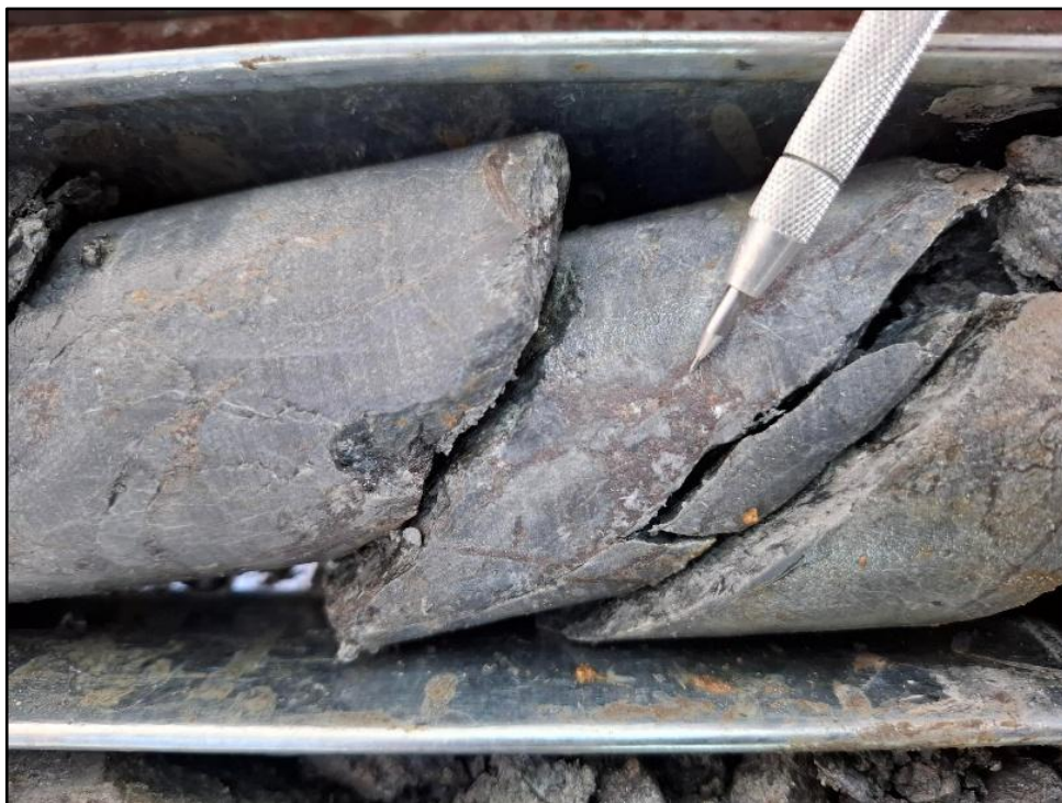
Figure 6. Core photo showing carbonate replacement pyrrhotite-pyrite-sphalerite-galena mineralisation in ZRPD25006 from 485.5 to 487.0m – 0.3% Pb, 2.2% Zn, 2.8g/t Ag.
