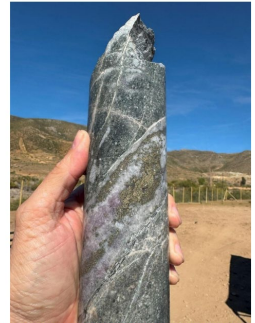
Photo 3 Anhydrite-pyrite-quartz vein within altered porphyry in 25LLDD0070 from 640m*.
