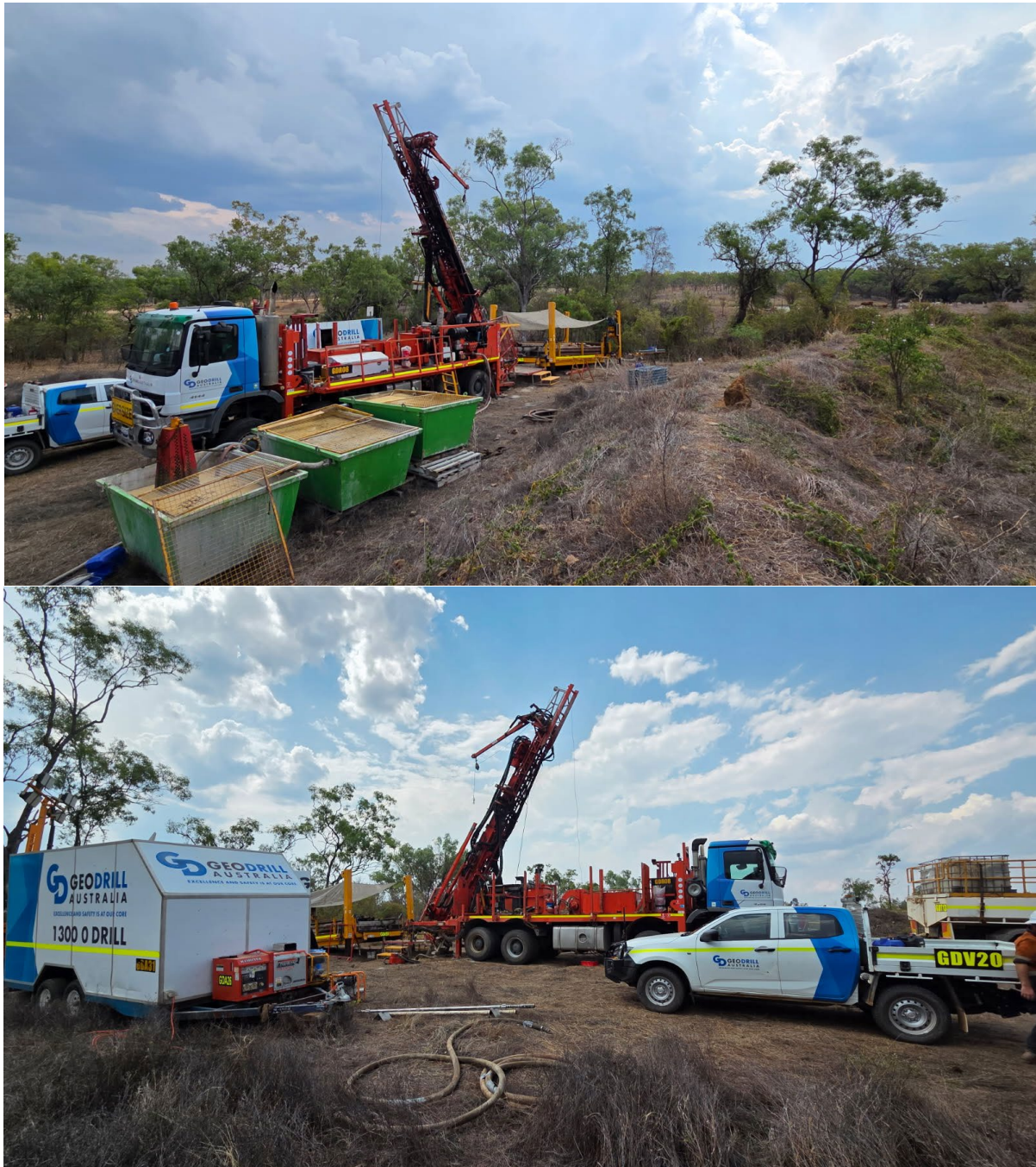
Figure 2: Diamond Drill rig set up on hole ELDD251016 at Electric Light
