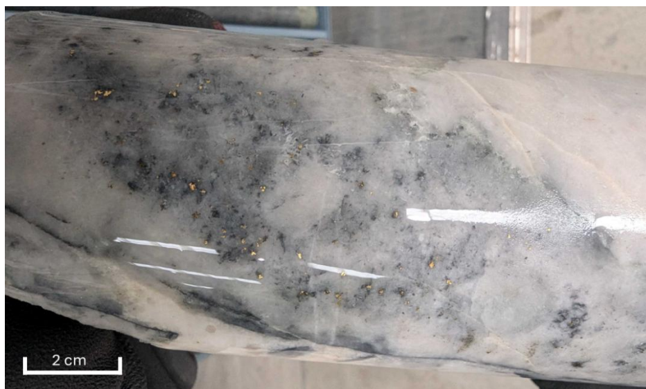
Figure 1: Visible gold in SDDSC208 showing quartz + carbonate + sulphosalts + stibnite, in 0.47 m downhole shear vein from 650.77 m (309 g/t Au & 0.03 % Sb) within a larger interval of 1.8 m @ 80.5 g/t AuEq (79.9 g/t Au, 0.2% Sb) from 649.4 m.
